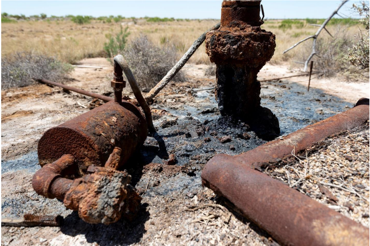
Figure 17. Oil field debris is often left behind and will be required to be removed as part of the methane leak plugging protocol.
