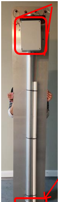
Capacitance Based Water Sensor ("Wet/Dry")
